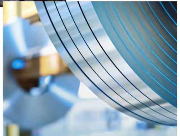
Non-grain-oriented electrical steel produced in Bochum is used in the manufacture of generators and electric drives.
