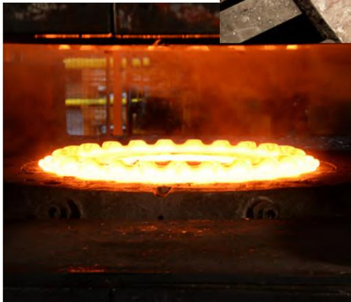
Forging a chainwheel for a mining excavator at Europe's largest forge press.
