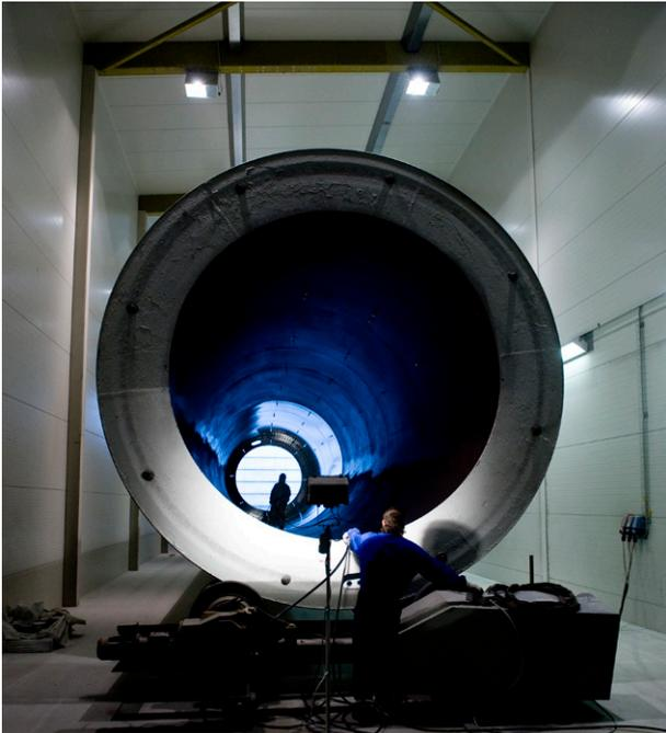
Surface coating of tower segments of wind turbines
